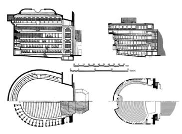
Figure 2 Plan and section<sup>5</sup> of Teatro Colon (left) and Dresden Semperoper (right) opera houses.
