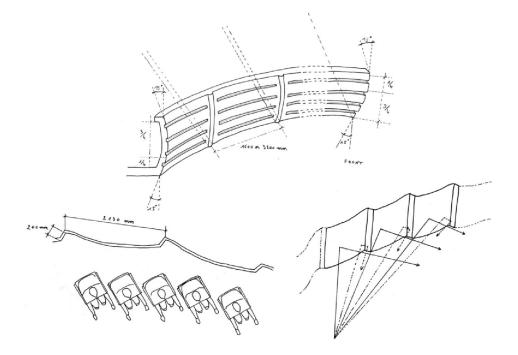
Figure 5 Acoustic sketches showing conceptual shaping for the walls and balcony fronts.
