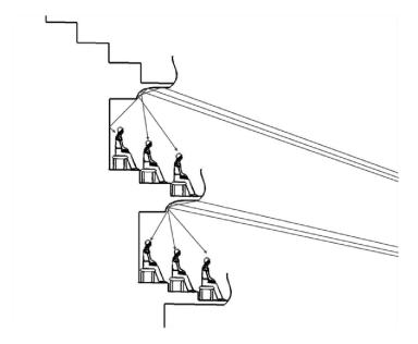
Figure 6 Acoustic sketches showing conceptual shaping for the balcony undersides.
